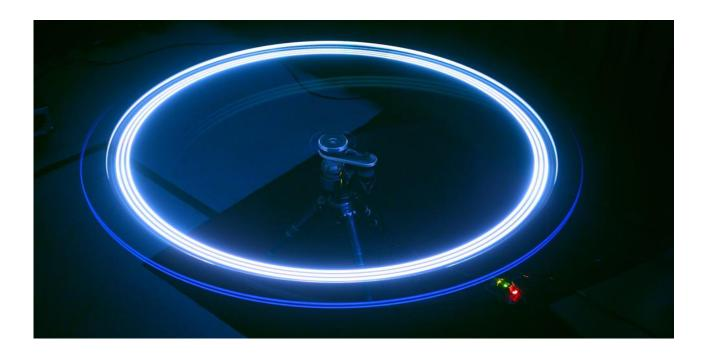
DR. DOPPLERS MACHINE explores spatialization using the Doppler Effect. The installation is a "persistence of hearing robot", think of "persistence of vision" (POV) and apply this to sound. It is a 2 meter wide spinning stereo speaker system in which sound fed in is distorted via the Doppler effect of speeds up to 500 rpm.
